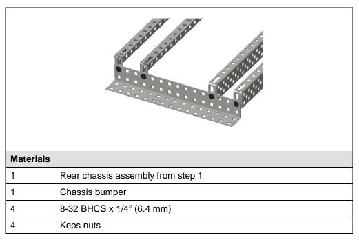
3 Make sure all of the components of the chassis frame are aligned and square, then tighten the hardware.
